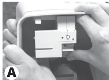
A. Align slot in Electronic Module with catch on back wall of dispenser housing and snap down into place behind left push tab.
