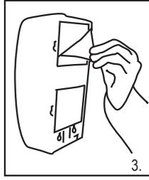
3. Remove the protective backing from the tape pads on the back of the dispenser. Carefully position the dispenser to the desired location and press firmly to the surface for 30 seconds.
