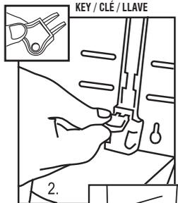
2. From INSIDE the dispenser, insert the key into the key slot located at the back of the dispenser and push until the latch piece is ejected from the bottom of the dispenser. NOTE: Place other hand under dispenser to catch latch piece.
