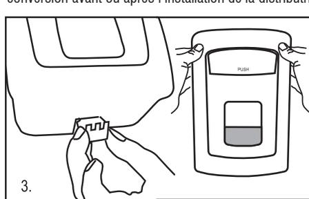
3. Re-install the latch piece in the bottom of the dispenser with the SLOTTED SIDE AWAY from the wall and toward the front of the dispenser. Push the latch piece into the dispenser until it snaps into place.
