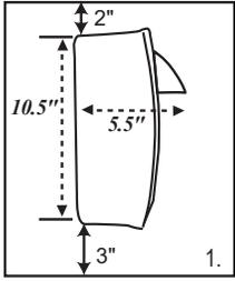
1. **IMPORTANT:** Dispenser opens to the front. For ideal placement, the dispenser should be mounted at least 3" above any countertop, fixture or obstruction and at least 2" below any upper cabinet, fixture or obstruction. \*See below for ADA guidance.
