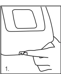
1. Open the dispenser by pushing up on the release latch. The latch is located on the bottom back edge of the dispenser in the center. While pushing the release latch, open the dispenser by placing your other hand on the top and guiding the front cover forward.
