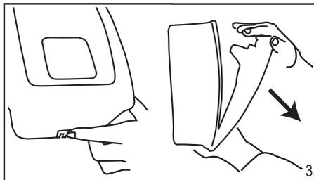
3. Open the dispenser by pushing up on the release latch. The latch is on the bottom back edge of the dispenser in the center.
