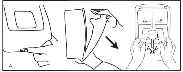
4. Open the dispenser by pushing up on the release latch. The latch is on the bottom back edge of the dispenser in the center.
