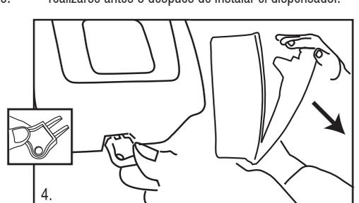
4. To OPEN, insert the key into the slots of the release latch on the bottom of the dispenser and push the key up. Place your other hand on top of the dispenser and guide the front cover forward. IMPORTANT: The dispenser can be converted back to the NO KEY REQUIRED mode. Complete steps #2 and #3 and insert latch piece with the SLOTTED SIDE TOWARD THE WALL.
