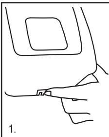
1. Open the dispenser by pushing up on the release latch (or with the key if you have converted the dispenser to the keyed locking mode). The latch is on the bottom back edge of the dispenser in the center. While pushing the release latch, open the dispenser by placing your other hand on the TOP, and guiding the front cover forward.
