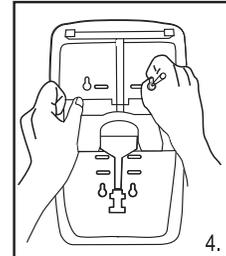
4. Hold the dispenser against the wall in the proper position and mark the appropriate slots. Set aside and drill holes in marked slots. Attach dispenser to the wall with the wall anchor and screws provided. You may choose to remove a portion of the protective backing from the tape to help hold the dispenser in position as you complete the installation.
