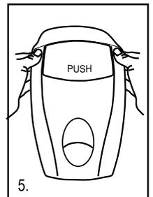
5. Close the dispenser: swing up front cover, then push on both sides at top with thumbs as shown. Push with even pressure until tightly closed. **DO NOT CLOSE BY PUSHING ON PUSH PAD!**
