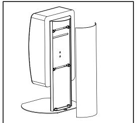
Mount back cover to stand by inserting one side into the angled flange and flexing the other side into place.
