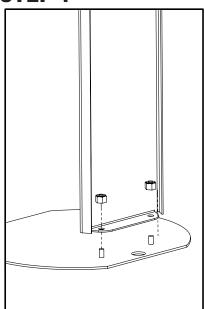
Attach column to base plate using two #8-32 Hex Lock Nuts.
