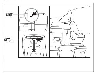
Insert electronic module by tucking the slot under the back catch and snapping down into place. Load refill bag bottom first and close dispenser.
