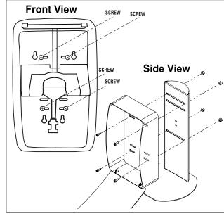
Align upper and lower mounting slots with slots in column. Fasten dispenser to stand using four #8-32 x 1/2" screws and #8-32 Hex Lock Nuts as shown.
